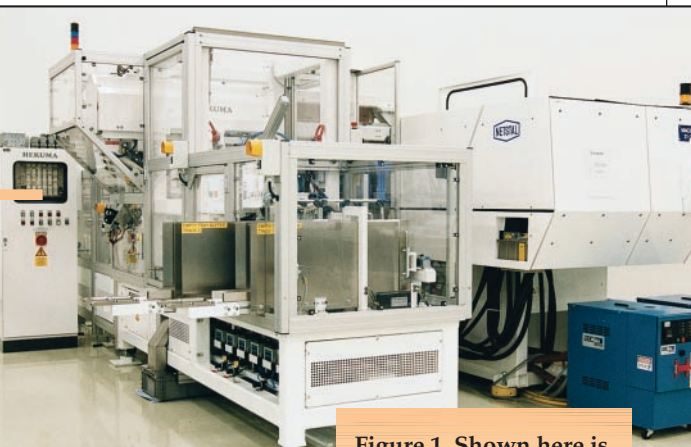
Figure 1. Shown here is a fully automated production system for Johnson & Johnson's Gemini Wells blood analysis system.
